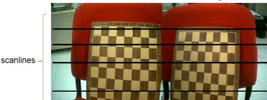
• Goal: transform the left and right image so that pairs of conjugate epipolar lines become **collinear** and parallel to one of the image axes (usually the horizontal one)
