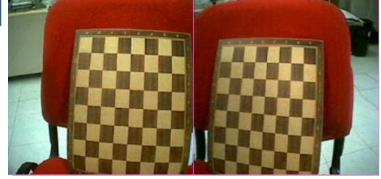
• Goal: transform the left and right image so that pairs of conjugate epipolar lines become **collinear** and parallel to one of the image axes (usually the horizontal one)
