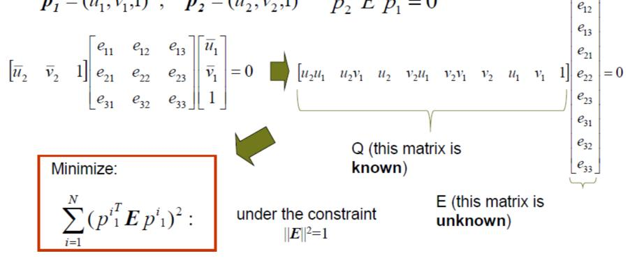
• A linear least-square solution is given through Singular Value Decomposition by the eigenvector of Q corresponding to its smallest eigenvalue (which is the unit vector that minimizes  $|Q \cdot E|^2$ )
