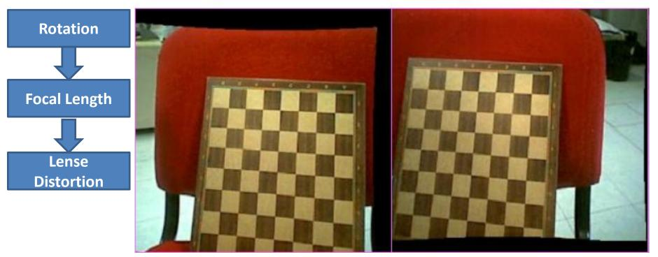
• Goal: transform the left and right image so that pairs of conjugate epipolar lines become **collinear** and parallel to one of the image axes (usually the horizontal one)
